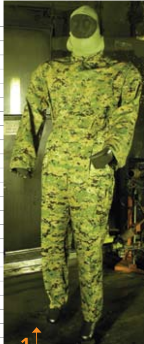
1 In a test performed at the request of the U.S. Marines, DriFire garments were exposed to an 850-degree direct flame for 3.5 seconds. (Garment shown prior to fire.)
