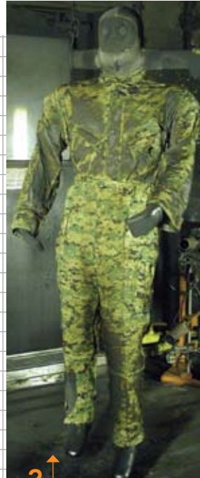
2 The outer garment was allowed to burn until the flames burned out (approximately 45 seconds). The test proved that DriFIRE was self-extinguishing. (Garment shown after flames burned out.)
